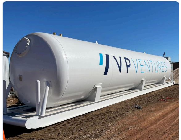
18,000-gal skid tank staged on roll-on / roll-off frame.
