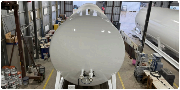
30,000-gal skid tank staged on roll-on / roll-off frame.
